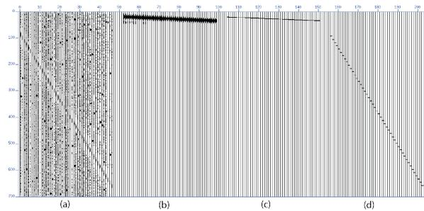
Figure 3: Steps of algorithm: (a) envelope; (b) SVD filtering after LMO correction; (c) picks determination; (d) inverse LMO and repositioning of picks on correct samples.
